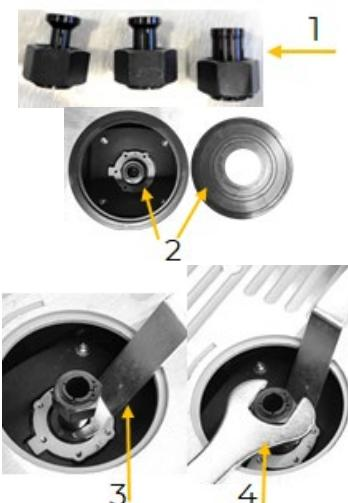
Select the collet ( $\varnothing$  6 mm,  $\varnothing$  8 mm or  $\varnothing$  12 mm) that corresponds exactly to the diameter of your milling cutter (1). Move the spindle to the highest position using the handwheel.
